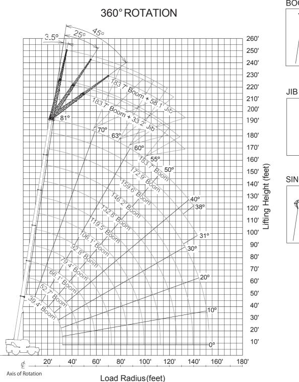
NOTE: Boom and jib geometry shown are for unloaded condition and machine standing level on frm supporting surface. Boom deflection and subsequent radius and boom angle change must be accounted for when applying load to hook. BOOM
